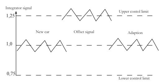
The amount of  $\lambda$  integrator offset is calculated when the set  $\lambda$  is equal to 1 and the canister close valve is closed.
