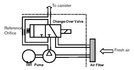
Leakage diagnostic (LD) is performed in after run mode, when key off.
