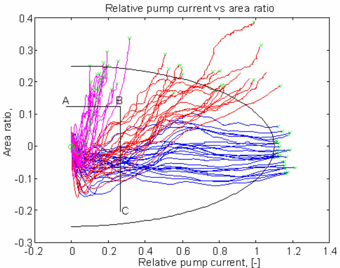
Results from simulation using old measurements and creating the area ratio and relative pump current and plot them versus each other.
